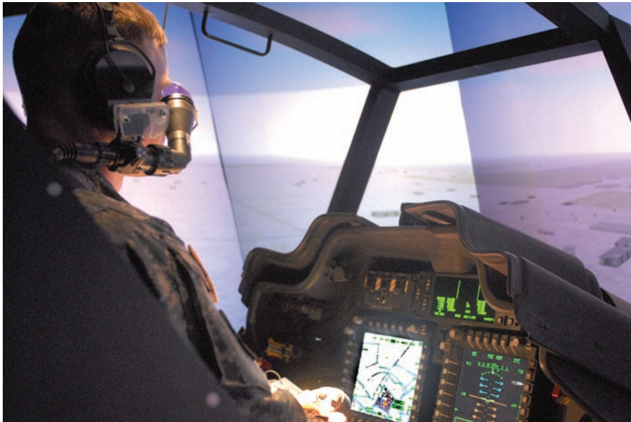
Fig. 2. An Apache attack helicopter pilot engaged in a simulated mission using a Longbow Crew Trainer located in a combat zone. [U.S. Army photo/Sgt. Brandon Little. Image provided courtesy of the U.S. Department of Defense Office of Public Affairs through the Digital Video and Imagery Distribution System]
